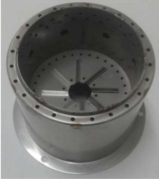
The image shows the new combustion tube model. It is a cylindrical metal component with a central vertical passage. The inner surface of the tube is lined with a series of shorter, straight vanes that extend from the center towards the outer wall, creating a wider, more uniform channel for the flame. Additionally, there are several small circular holes around the inner circumference of the tube. |
